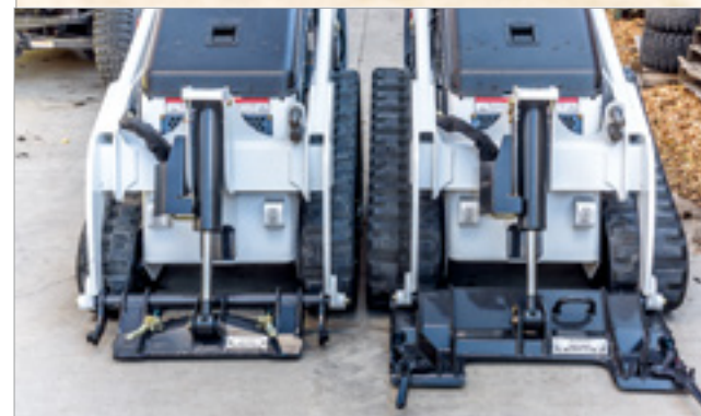
COMMON INDUSTRY INTERFACE BOB-TACH ATTACHMENT MOUNTING SYSTEM
